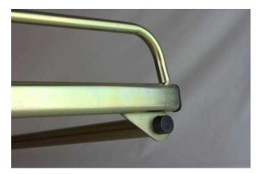
...and fit the roller at the back as you install the other side. The bearings are made from self-lubricating Nylotron (graphite impregnated nylon) and need no additional lubrication.
